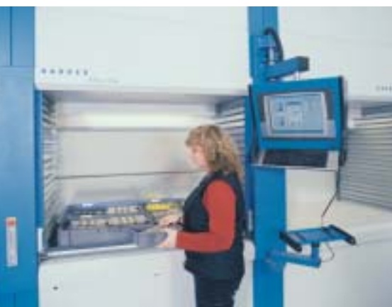
The tray containing the requested articles is made available at the press of a button and automatically takes the fastest and shortest route.
