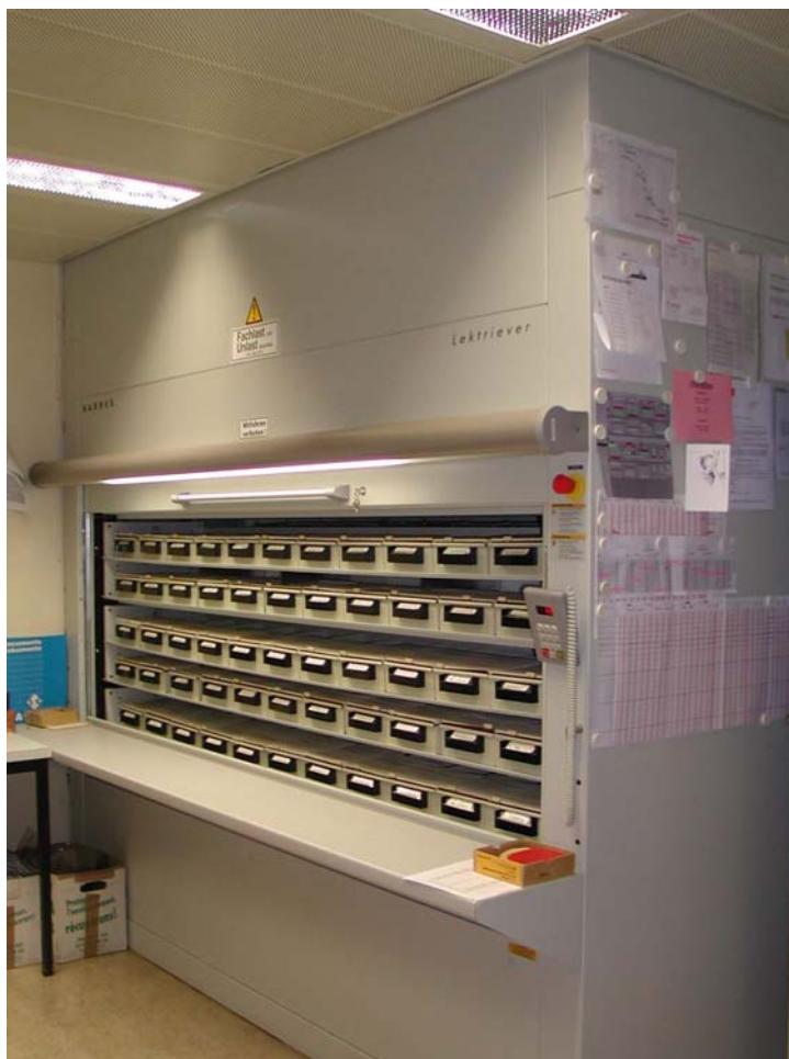
Lektriever® 120/19-12", Dimensions: 2560 x 3500 x 1155 mm (BxHxT) 38 Levels with 11 cassettes each, ca. 770'000 microfilms
